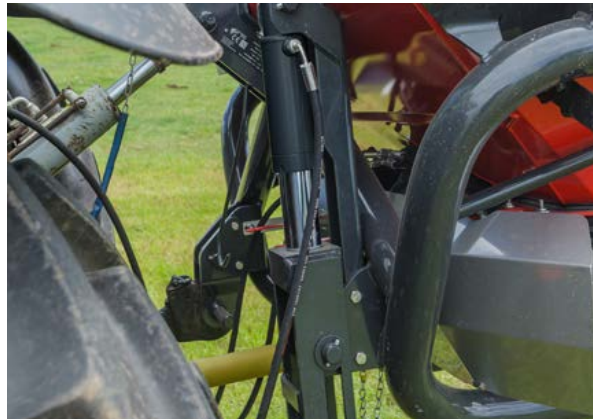
Border spreading with tramline cylinder - spreading towards the border from the last tramline
