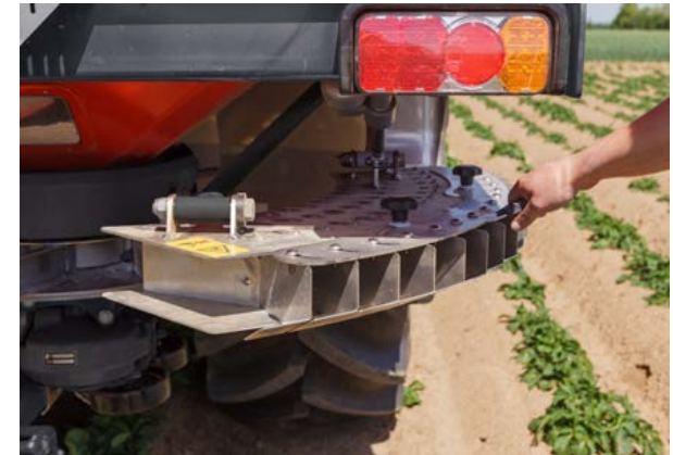
Border track spreading - spreading to the border with the ExactLine
