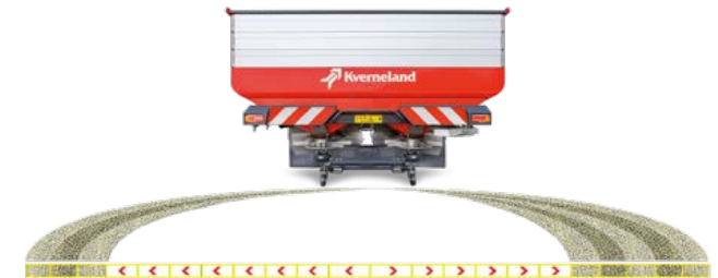
Switching off the sections outwards
